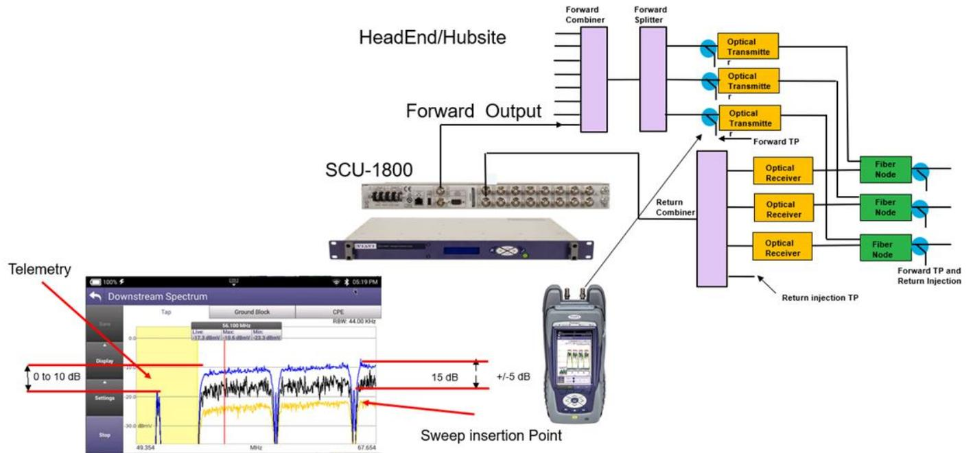
Figure 3: Forward Telemetry Placement and Level test point
