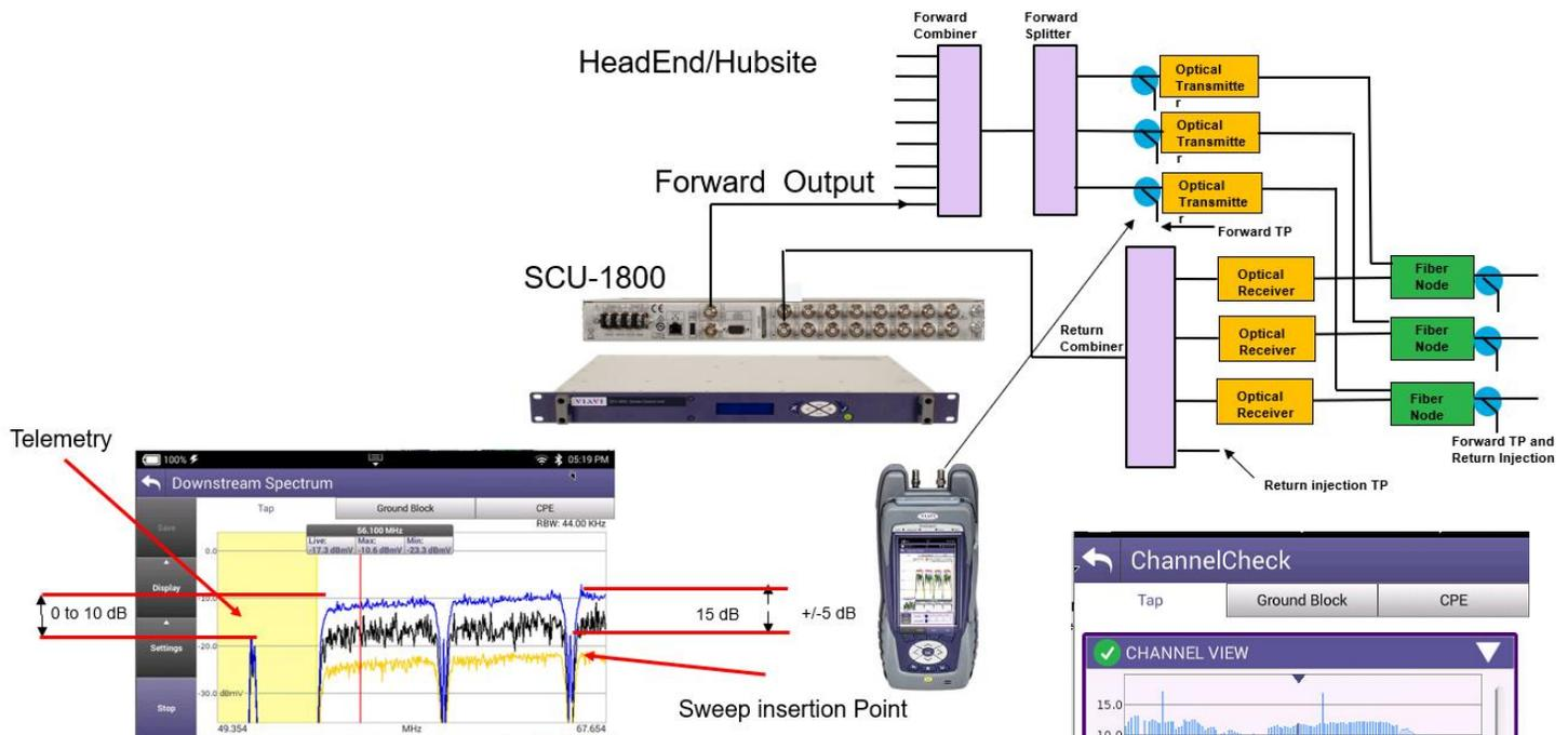
Use Channel check to verify no BER errors and DQI level less than 10
